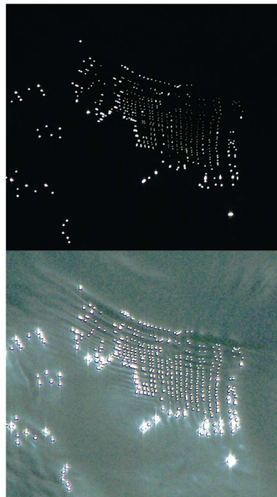
Fig. 6. (Color online) Top: image of resolved glitter adjusted to show only the glints. Bottom: same image adjusted to show the glints and the water's surface (ocean).
