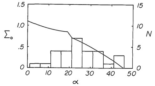
FIG. 4. Comparison of observation  $[N(\alpha)]$  and theory  $[\Sigma_0(\alpha)]$ . The thick curve shows  $\Sigma_0(\alpha)$  the total relative cross section as a function of  $\alpha$ .  $\Sigma_0 = \sigma_0 + \sigma'_0$  below  $19.08^\circ$  and  $\Sigma_0 = \sigma_0$  above it. The right-hand ordinate is  $N(\alpha)$ , the histogram of anthelion counts as a function of  $\alpha$  in  $5^\circ$  bins. Both  $N(\alpha)$  and  $\Sigma_0(\alpha)$  go to zero near  $46^\circ$ .
