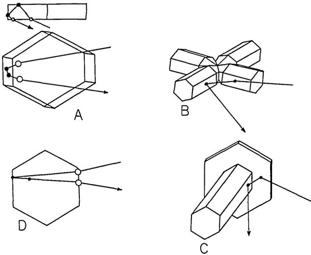
FIG. 1. Anthelion-producing mechanisms. The dots show reflections and the circles show transmissions. A, Bravais; B, Besson; C, Humphreys; D, partial contributor to the mechanism proposed in this paper.
