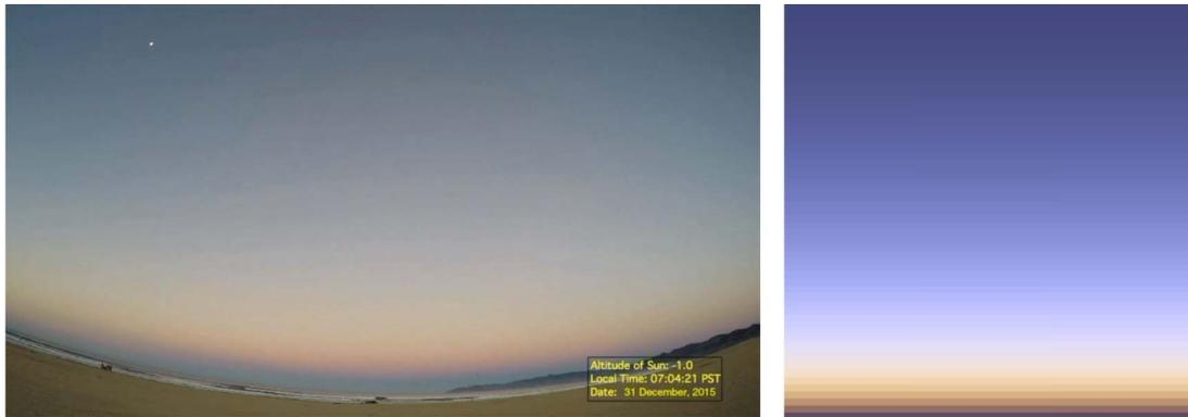
**Fig. 1.** Video frame (left) and MCScene simulation (right) comparison for  $\epsilon = -1^\circ$ .
