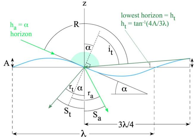
Fig. 3. Optical geometry of Snell's window in the presence of surface waves.
