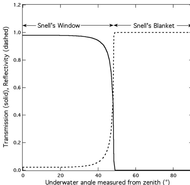
Fig. 6. Transmission of flat water producing Snell's window (solid line) and reflectivity of the under surface of water producing Snell's blanket. The angle from zenith is what an underwater observer would measure.
