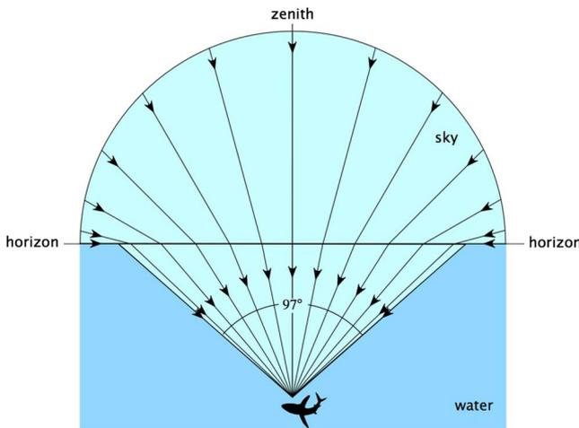
Fig. 2. Optics of Snell's window for flat water.
